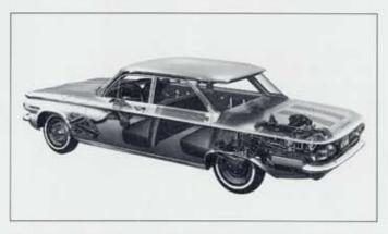
As a result, compact cars arrived from the "Big Three" in late '59 as '60 models. The Chevy model was the Corvair, an innovative departure from the crowd. Powered by an air-cooled, rear-mounted 6-cylinder engine (the first air-cooled Chevy since the mostly experimental 1923 copper-cooled Chevrolet), Corvair was available in three styles — base "500" Coupe and Sedan, mid-level "700" and the mid-year "900" Monza Coupe.
