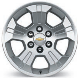
18" Bright Machined-Aluminum (Standard on LT Z71 and LTZ Z71)
