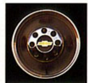
Standard 16" wheel for 3500 Series when equipped with dual rear wheels.
