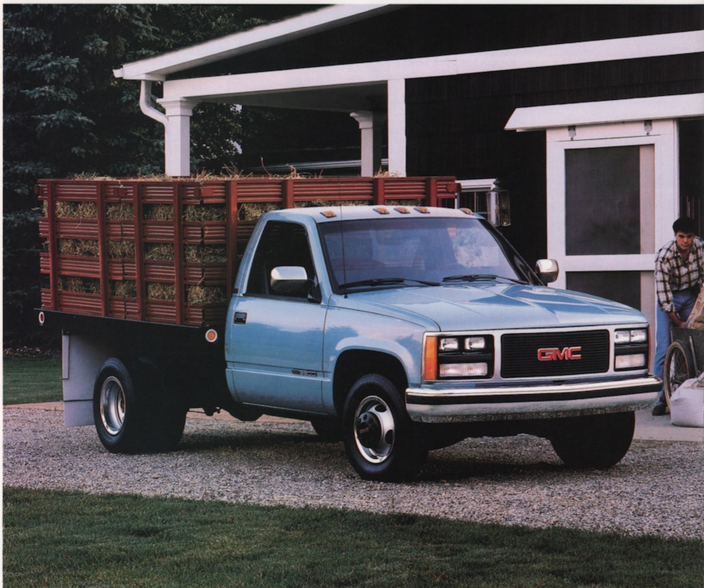
2-WD Sierra Series C-3500 Cab & Chassis shown with dual rear wheels and other available equipment, including stake rack body from outside supplier
