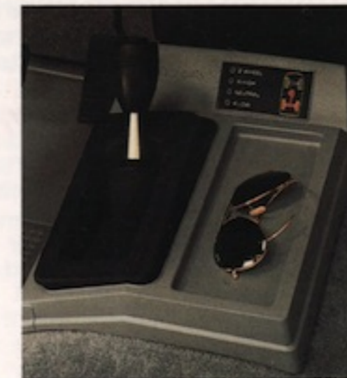
Single-lever Insta-Trac transfer case control allows you to shift from 2 WHEEL to 4 HIGH and back, at any speed. A lighted display indicates your driving mode.
