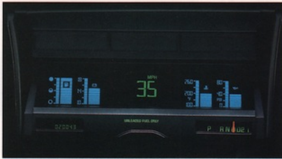
Electronic instrumentation has tachometer and gages with vacuum fluorescent displays.
