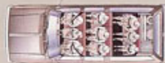
9-person arrangement with standard front bench seat and available center and rear bench seats
