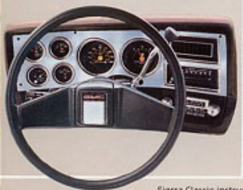
Sierra Classic instrument cluster with needle-type gauges to indicate charging system voltage plus engine temperature and oil pressure
