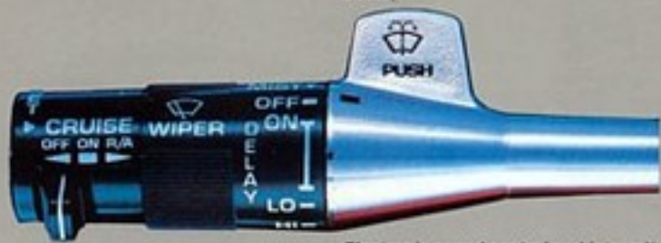
Electronic speed control and intermittent wiper shown on standard multi-function switch.
