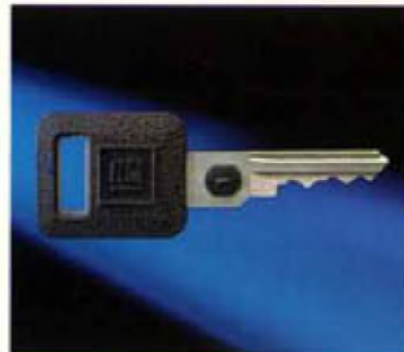
VATS EMPLOYS A DECODER AND IGNITION KEY WITH A PELLETT OF SPECIFIED RESISTANCE.
