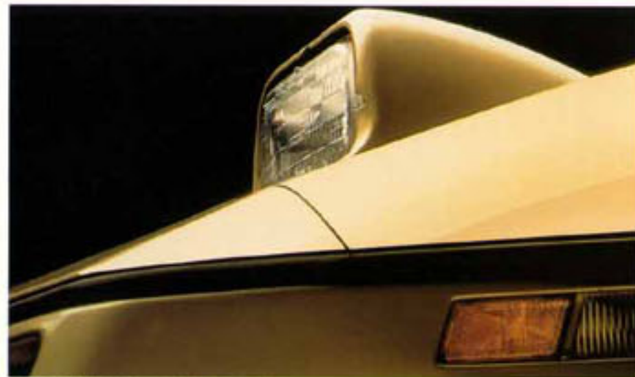
RETRACTABLE HEADLAMPS FLIP FORWARD 162.5 DEGREES FROM BENEATH THE HOOD.
