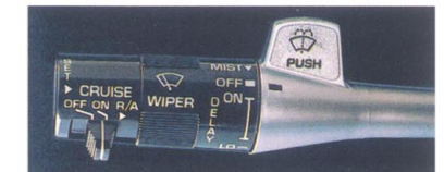
Electronic speed control and intermittent wiper control on standard multifunction switch
