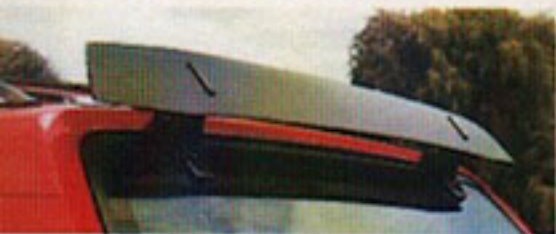
Roof air deflector
