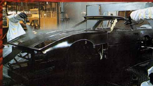
Robot painters apply base coat.
