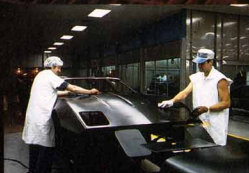
Meticulous wet and hand sanding are demanded by Corvette's tough paint inspection standards.
