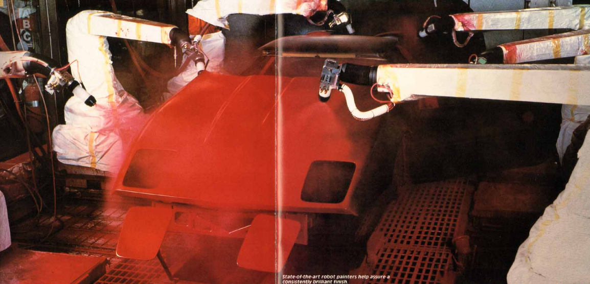
State-of-the-art robot painters help assure a consistently brilliant finish.
