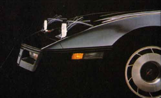
Powerful electric motors rotate the headlamps.
