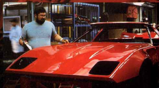
Meticulous wet and hand sanding are demanded by Corvette's tough paint inspection standards.
