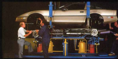
Specialty built hydraulic towvever system "marries" chassis to body.
