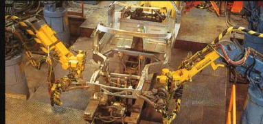
Uniframe components get additional precision robot welds.
