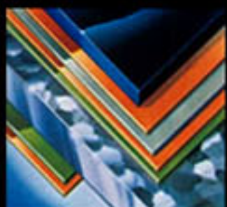
Lower fender cross section shows layers of corrosion protection including galvanized Zincrometal ® , zinc-rich primers and anti-chip Plastisol.
