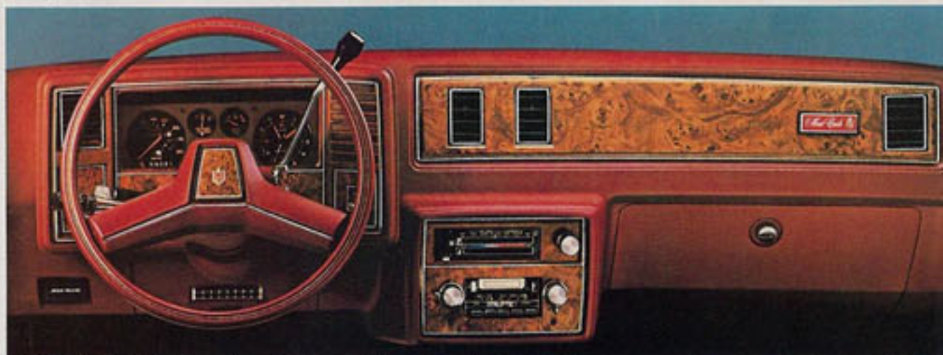
Monte Carlo instrument panel shown with optional gauge package. NOTE: Speedometers in Canada have major scale in km/h, secondary in MPH and odometer in kilometres.
