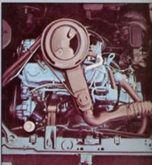
Standard 2.5 Liter 4-cylinder engine is rated 90 hp and is transverse-mounted over the front wheel drive.
