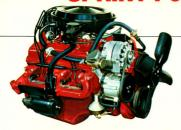
Sprint power starts out with a standard 2-bbl. 350 CID. V-8 engine and advances to the available 400 or 454 CID, V-8 engines for a blend of durability and responsive performance, GMC V-8 engines provide good performance and operating features. Hardened valves contribute to durability. Cooling around cylinders helps maintain uniform temperatures. Pressure Jubrication provides oiling of internal moving parts and helps lower operating temperature.
