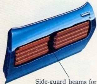
Side-guard beams for side impact protection.
