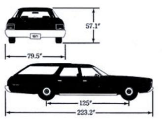
Tailgate opening height 29.5" Tailgate opening width at floor 48.8" Tread, front 64.1" Tread, rear 64.0" Standard tire size L78-15 Rated fuel tank capacity 24 gal. Load floor length 100.5"† Total cargo volume 106.4 cu. ft.
