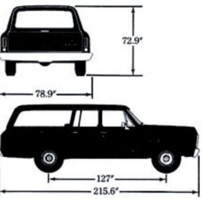
Tailgate opening height 40.7" Tailgate opening width 57" Tread, front 64.1" Tread, rear 62.7" Standard tire size G78-15 Fuel tank capacity 23.5 gal. Load floor length 114"† Total cargo volume 181.3 cu. ft.
