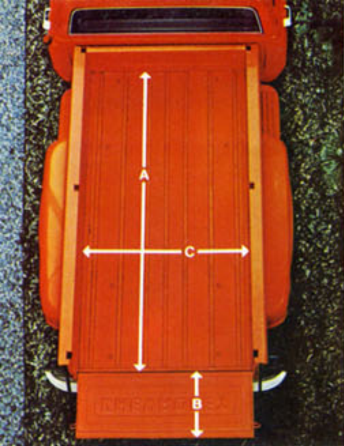
Wood Floor with Steel Skid Strips
