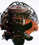
The standard engine you get is a 300-horse 350-cubic-inch V8 that inhales through 4-barrel carb and exhales through dual exhausts. If you want still more, you can order the 350-horse 396-cubic-inch V8. When you order this big one you get a special suspension with a rear stabilizer bar. Both engines require 4-speed or Turbo Hydra-matic. That way you've got all the horses in the palm of your hand.
