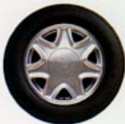
Standard 16" x 7" squeeze-cast aluminium wheel
