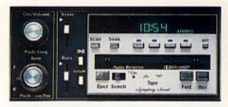
Delco-GM/Bose Symphony Sound System. Standard on Allanté. Cadillac's ultimate stereo is customized to the exact dimensions and acoustical characteristics of your Cadillac. Includes four separate amplifiers and speakers, each in its own special enclosure. (Four amplifiers in the trunk on Cimarron.) Also includes Integral Cassette Tape Player with Auto Reverse, Tape Equalization, Dynamic Noise Reduction (DNR\*), Dolby\* Tape Noise Reduction, Full-Time Loudness Control and more.
