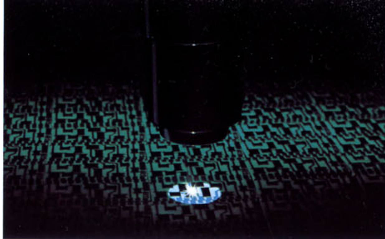
Laser trimming of Electronic Control Unit for Cadillac's exclusive Electronic-Fuel-Injected Engines.
