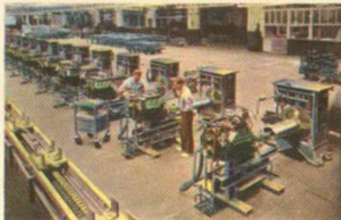
Engines are run continuously for many hours. Smoothness, quietness, and compression are checked and rechecked by accurate machines.
