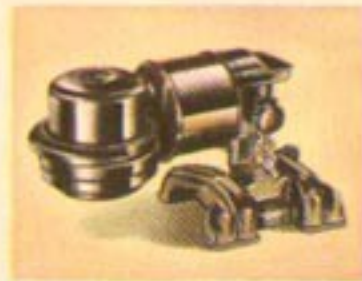
Dual intake manifolds reduce gasoline condensation and assure equal fuel distribution to all cylinders.
