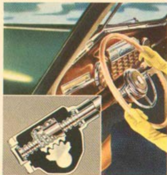
The ball bearing steering gear, stronger than conventional assemblies, gives Cadillac cars unexcelled steering ease.
