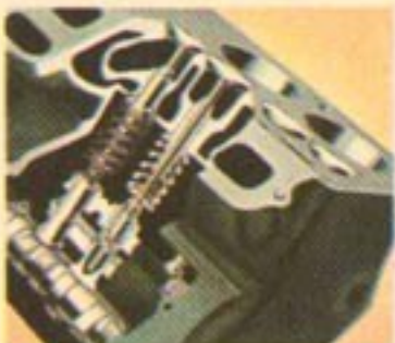
Hydraulic valve silencers assure efficient fuel consumption by maintaining accurate valve seating.
