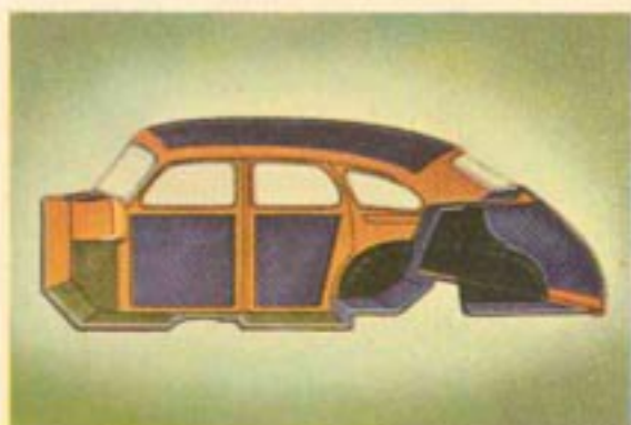
Body insulation, further improved this year, results in a noticeably quieter body. Six insulating materials are used.
