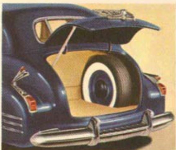
Pictured is the spare wheel mounting in trunk and the concealed gas tank filler cap under left tail light.
