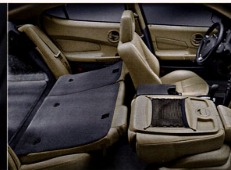
Fold-flat rear seats and front-passenger seat
