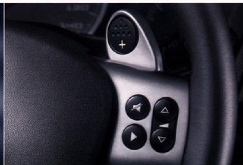
TAPshift – steering wheel-mounted shift paddles
