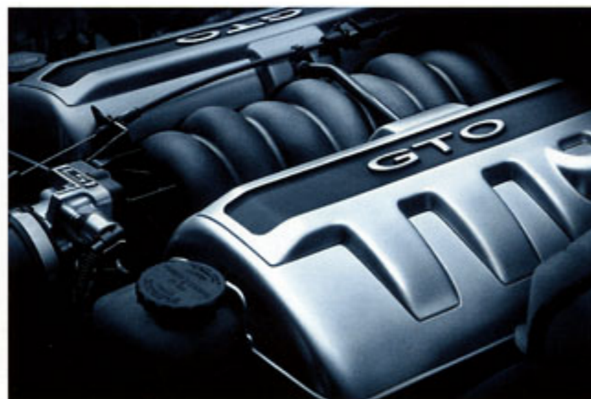
Gen III LS1 V8 engine with 350 horsepower
