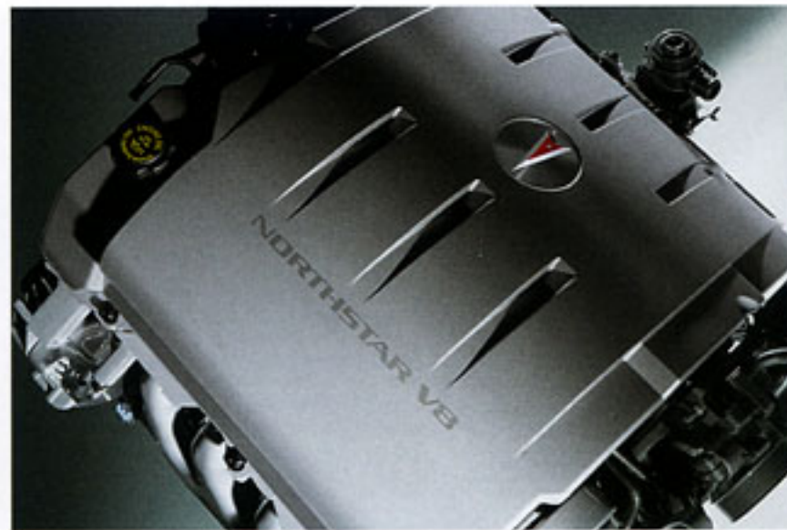
275-hp 4.6L Northstar V8 engine
