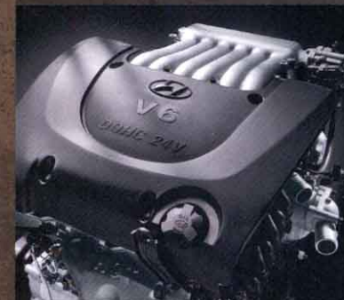
The 2.7-liter aluminum DOHC V6 engine, standard on Santa Fe GLS and LX delivers dependable performance with minimal scheduled maintenance.
