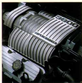
The available supercharged 3800 V6 engine boosts peak output to 225 hp and 275 lb-ft torque.
