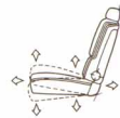
The available six-way power driver's seat has fingertip controls, located on the front of the seat.
