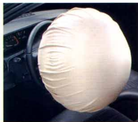
A standard driver air bag, used with three-point safety belts, can help prevent injury in certain severe frontal impacts.
