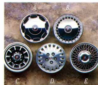
A. 14" Styled Chrome Wheelcovers B. 14" Deluxe Chrome Wheelcovers C. 14" Styled Steel Wheels D. 14" Aluminum Wheels E. 14" Custom, Locking Wire Wheelcovers
