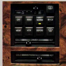
The dual ComforTemp climate control available in Regal lets you and your front-seat passenger select separate temperature settings.
