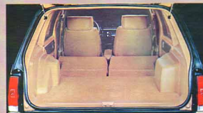
With the rear seat down, there's 63.4 cubic feet of carpeted cargo area.
