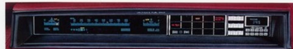
Enjoy the advanced technology of an available electronic instrument panel. It includes multicolor vacuum fluorescent display of vehicle speed, fuel level, engine temperature and trip odometer. Voice information reminder system is also available.
