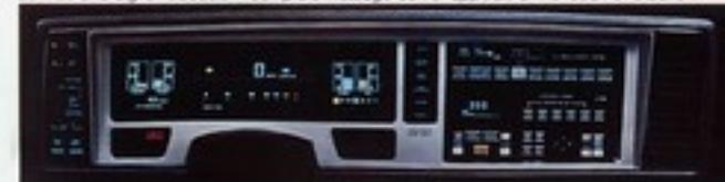
Multicolor displays feature easy-to-read shapes, lighted push-button controls and digital readouts. A complete message center appears at the touch of a button.
