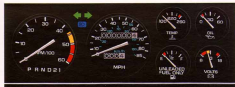
Rallye instrument panel cluster. Includes: tachometer, trip odometer, voltmeter and temperature and oil pressure gauges.
