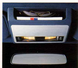
Header-panel mounted courtesy lamp is standard and features an integral storage compartment for convenience.
