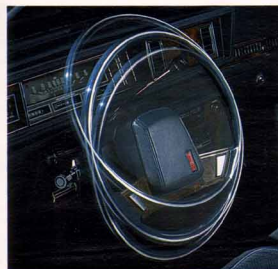
Tilt-Wheel steering. Adjusts to six different driving positions. Swing up for easy entry and exit.
