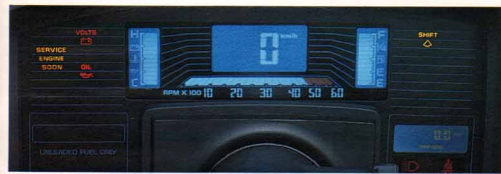
Optional Electronic Instrument Cluster offers the newest technology in electronic instrumentation and features a multiple color crystal (LCD) display that doesn't "wash-out" in daylight. Cluster includes center-mounted digital speed readout, analog bar graph tachometer, animated warning lights and a selectable multifunction gauge for voltmeter, oil pressure and temperature.
