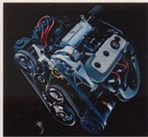
3.8-liter V6 with sequential port fuel injection.
