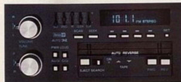
ETR AM/FM stereo with seek/scan, digital clock, dual rear speakers
