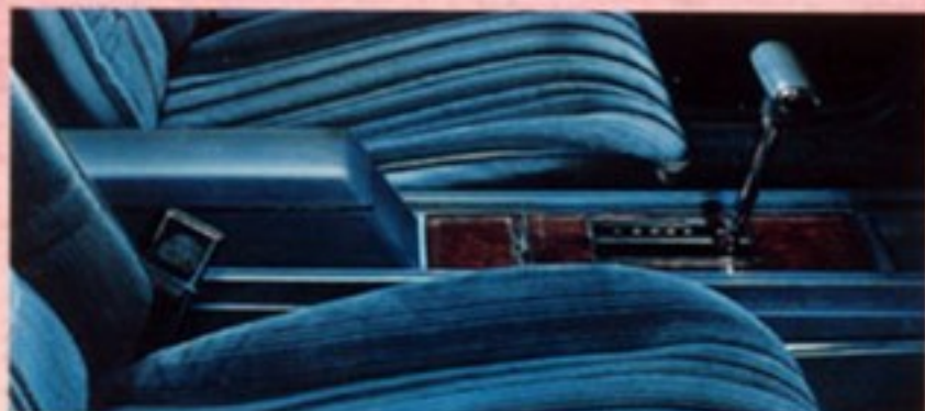
Floor-mounted console shifter, available. If you like the look and feel of bucket seats, add to it with this sporty floor-mounted automatic shifter (standard on Cutlass Salon).
