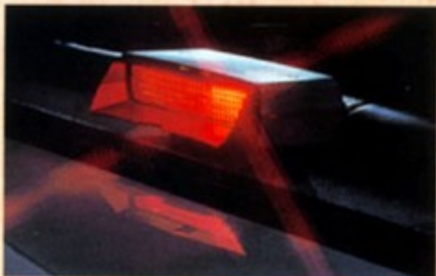
This new high-level stoplight is mounted behind the rear window. Just step on the brake pedal and it lights up at the same time as the rear tail lamps.
