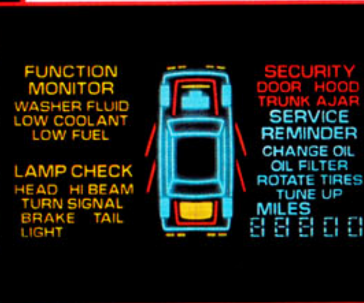
The STE's Driver Information Center keeps track of important mechanical functions, fluid levels and maintenance intervals.
