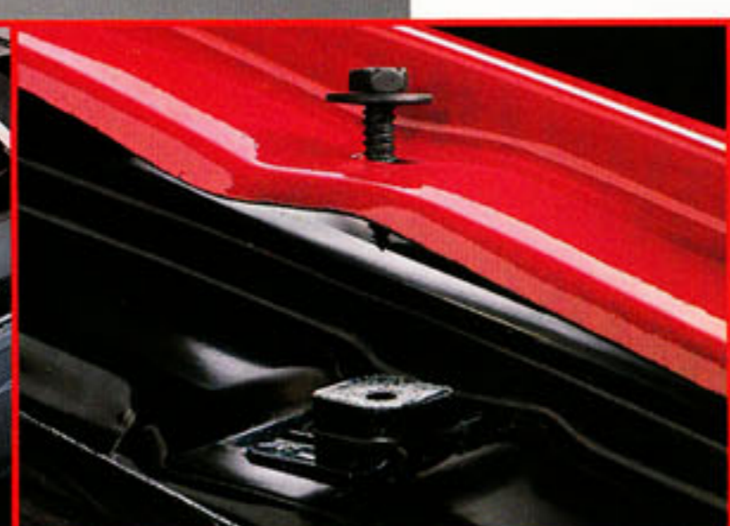
In yet another innovative approach, the Enduraflex™ panels are mechanically attached to the space-frame.
