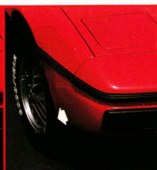
The front fenders actually bounce back from minor impacts, and the other panels resist minor dents and dings.
