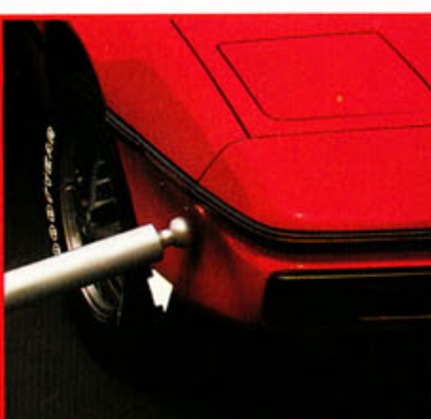
The front fenders actually bounce back from minor impacts, and the other panels resist minor dents and dings.
