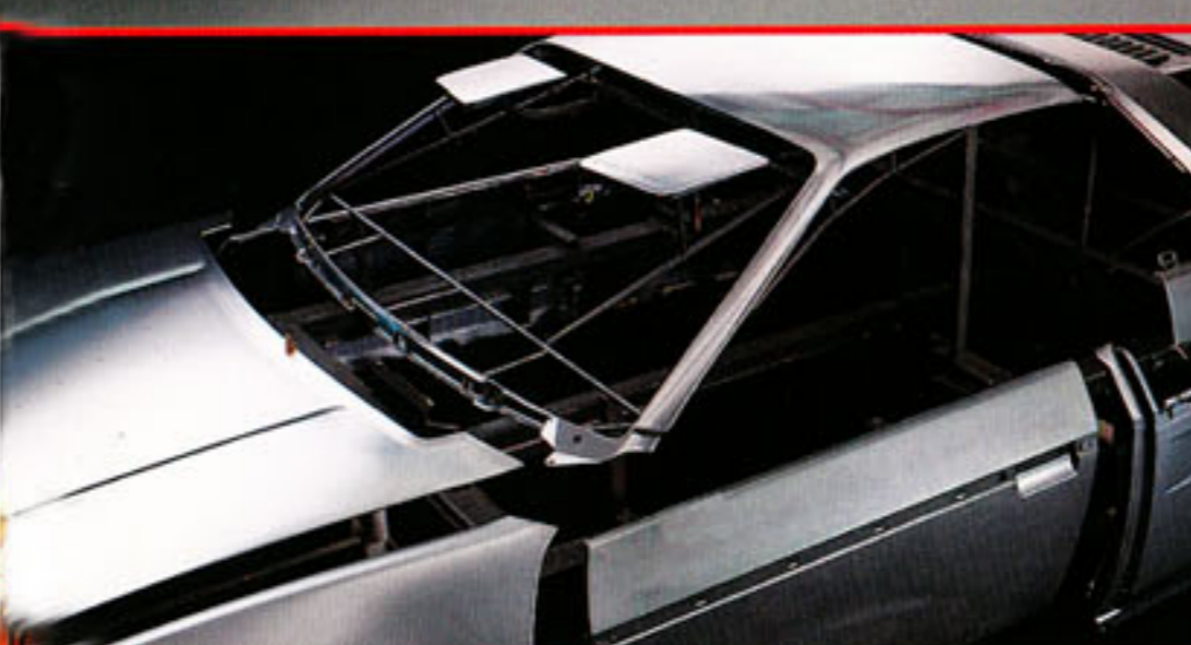
ENDURAFLEX™ panels are loaded on a floor-mounted carrying fixture in an "in car" position for painting.
