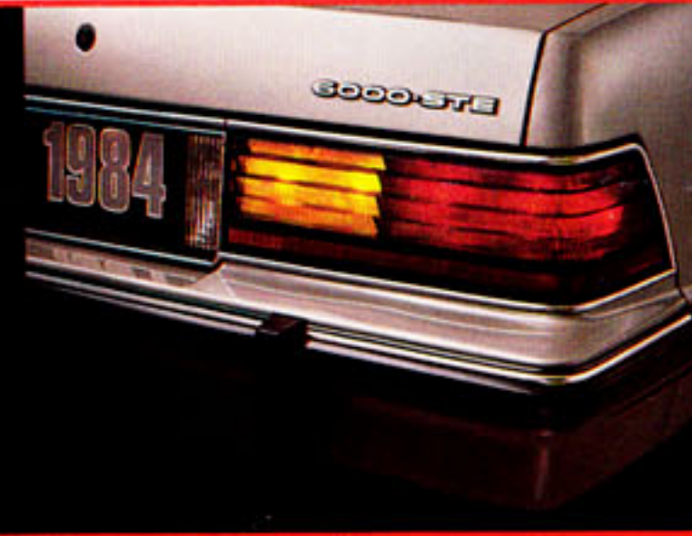
The STE's new neutral-density taillight includes amber lens turn signals.
