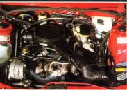
Spotts-car pickup and miserly fuel efficiency start here. The optional 1.8 liter L4 overhead cam power-johnt is perfectly matched to the 5-speed overdrive manual transmission for mileage, dependability, and a respectable amount of "zip." You can also order the 1.8 liter engine with the floor shift automatic.
