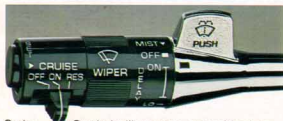
Cruise Control with resume-speed feature. Lets you select the cruising speed you want.
