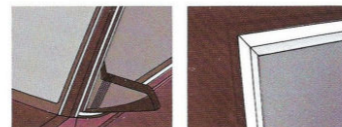
The one-piece flush-mounted windshield molding and tightly-butted window molding corners help give J2000 a clean appearance.
