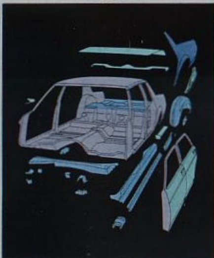
Extensive use of zinc-rich primers, wax sealers and anti-corrosion metals help provide extensive protection against rust.
