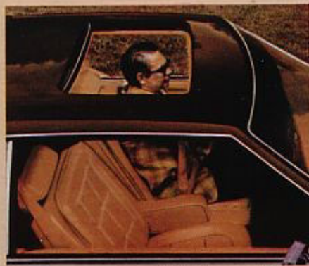
Electric sunroof is available in metal or tinted glass (reduces headroom slightly).
