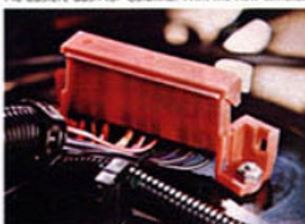
Diagnostic connector for electrical service.
