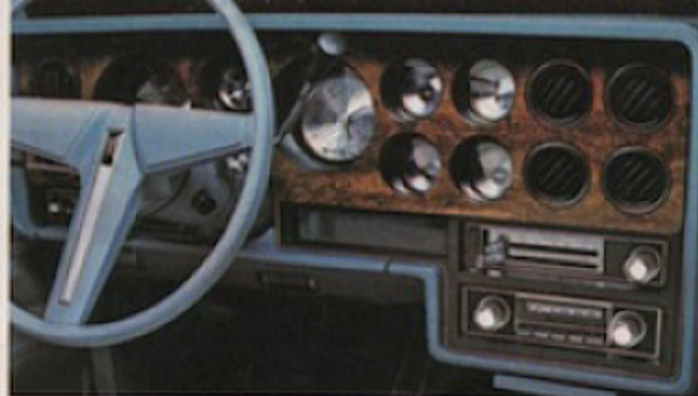
LeMans Safari's instrument panel was designed to be easy to service from the front.
