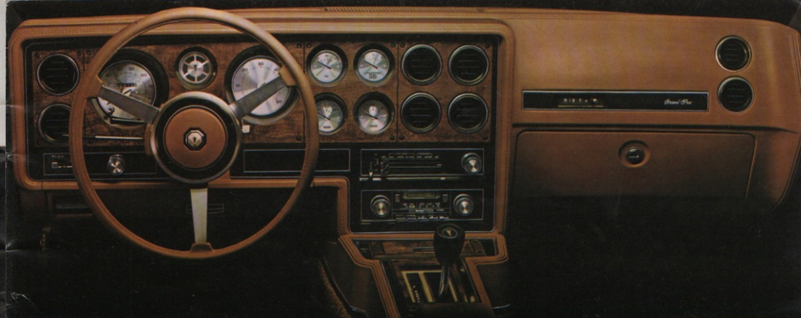
The new Grand Prix LJ instrument panel with available custom sport steering wheel and Rally gages.
