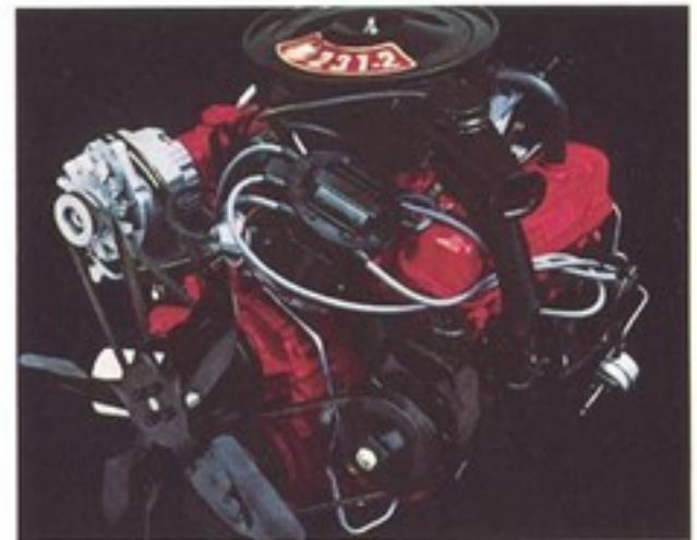
Skyhawk's new V6 231 CID engine
