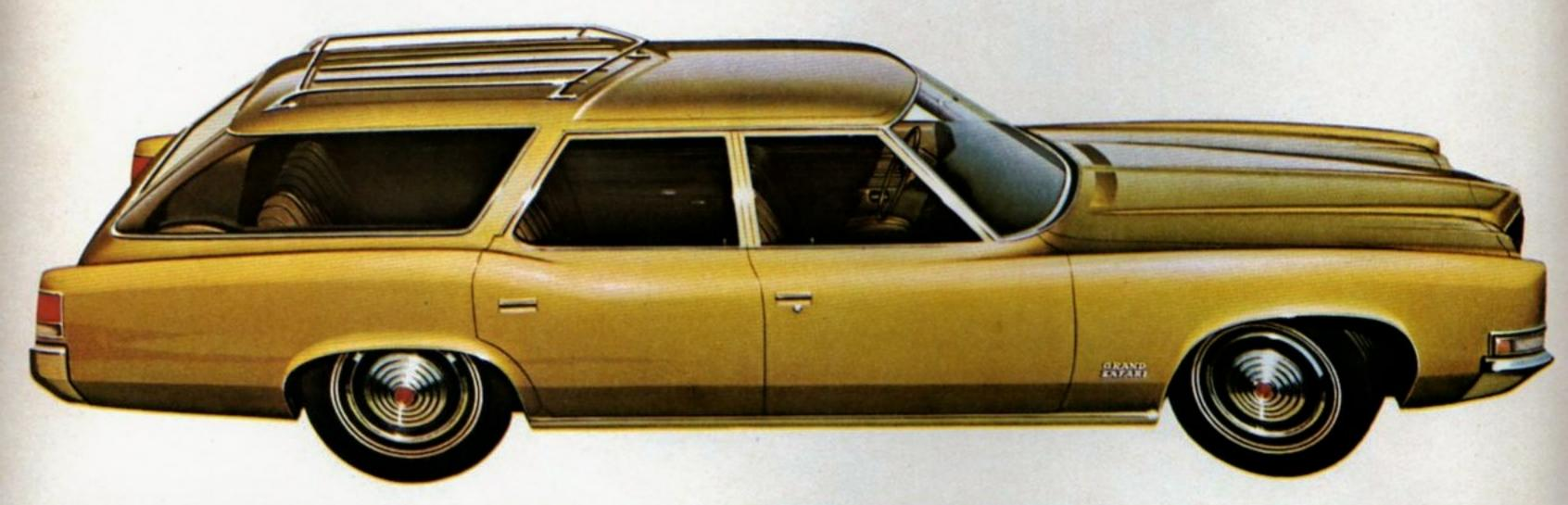
Typically, our chassis engineers were more than a little enthusiastic when they worked on handling this year. Which is why Grand Safari has power steering. A 1-1/8-inch stabilizer bar in the front. Power brakes with front discs and 12-inch drums in the rear. And, of course, Pontiac's Wide-Track stance.
