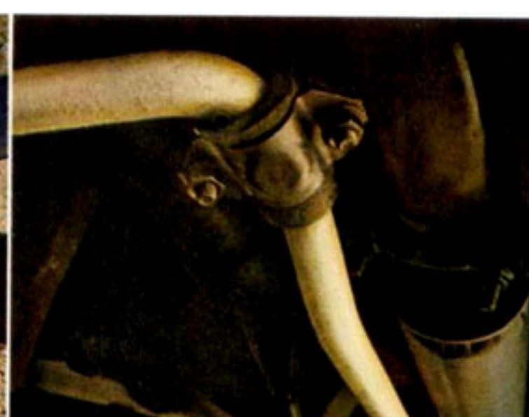
New rear stabilizer bar (5/8" diameter).
