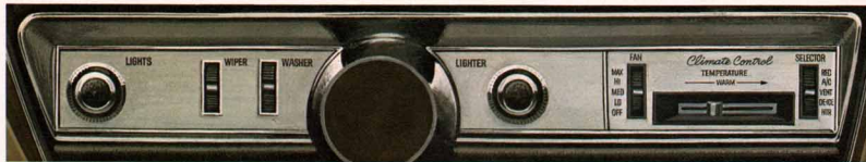
Here are just two more thoughtful touches from Buick for 1969. Selecting the right climate and temperature for your Sportwagon becomes easier than ever this year. The addition of new slide-operated controls for both heating and air conditioning units provides quicker, easier adjustment.
