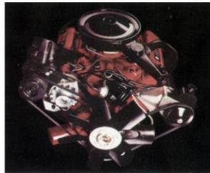
The 350-2 V8 engine. Another Buick powerplant that's new for '68. 350 cubic inches, 230 horsepower, 350 pounds feet of torque. Power, Economy, Dependability. Standard on the Special Deluxe 2-Seat Wagon, all Skylark Custom models, Custom Sportwagon and LeSabre. Available on Special Deluxe Coupe and Sedans, Skylark Sport Coupe and Sedan.
