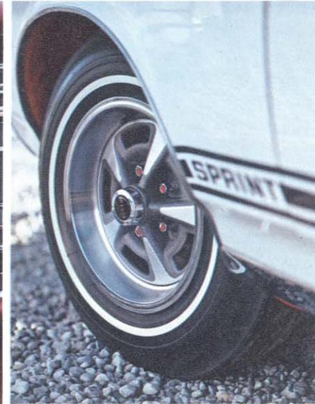
The Rally II wheel may be ordered with or without disc brakes.
