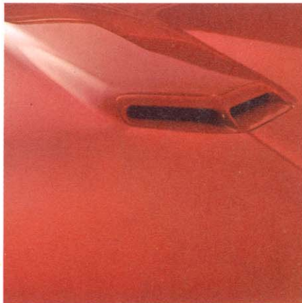
You can even order a special Ram-Air engine option that draws air through the scoop.
