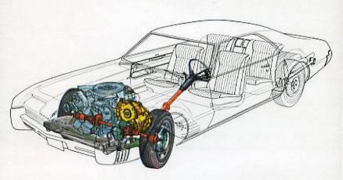
Front wheel drive puts the traction where the action is! Toronado Rocket V-8 feeds power to front wheels via Turbo Hydra-Matic. Result: Toronado pulls (rather than pushes) you through tightest turns. Improves traction and stability. Reduces vibration and noise.
