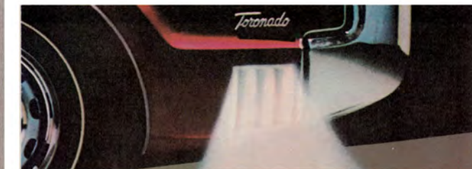
Take a corner with confidence! Cornering lights operate automatically when you use directional signals with lights on—assure more convenient turning at night.
