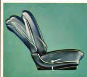
Reclining Seat —Adjusts as much as 30° up or down for passenger comfort. Available on Toronado Deluxe, Starfire and Cutlass; on Toronado, it is available when optional Strato Seats are ordered.
