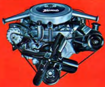
Toronado Rocket V-8. Oldsmobile's top-performing Rocket. Twin-snorkel air cleaner. Quadrajt Carb. 425-cu.-in. 385 hp. 475 lb.-ft. torque. 10.5-to-1 compression. Standard on both Toronado models.
