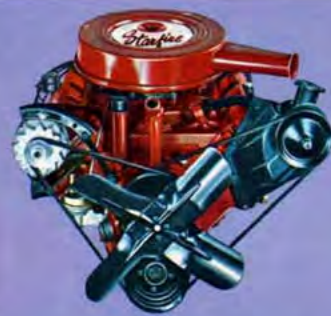
Starfire V-8. Quadrajt Carburetor. High-lift camshaft. 425-cu.-in. 375 hp. 470 lb.-ft. torque. 10.5-to-1 compression ratio. Premium fuel. Standard on Starfire. Optional on all Ninety-Eight and Delta 88 models.
