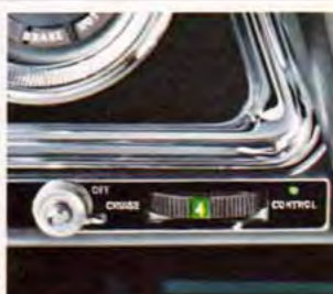
Cruise-Control —Set your speed and Cruise-Control maintains it, while reducing fatigue. Has built-in resistance when set speed is reached, acts as warning device. Extra cost option on all models.
