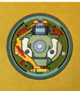
Air-Scoop Brakes have wide flange that sweeps up air to dissipate heat. Thick linings reduce wear. Large lining areas, plus organic compounds, aid stopping power. All brakes are self-adjusting, self-energizing.
