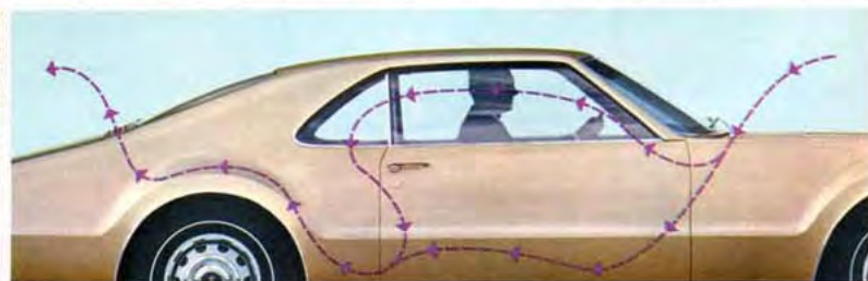
Unique new draft-free ventilation system brings outside air in at two levels through five adjustable outlets. Circulates air through car—without noise, without draft—and releases it through louvers below rear window. Makes conventional side vent windows completely unnecessary.
