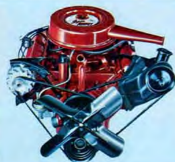
Super Rocket V-8. New 2-barrel carburetor. 310 hp. 450 lb.-ft. torque. 425-cu.-in. 10.25-to-1 compression. Premium fuel. Standard on Delta 88 and Dynamic 88. 300 hp regular fuel available, no extra cost.
