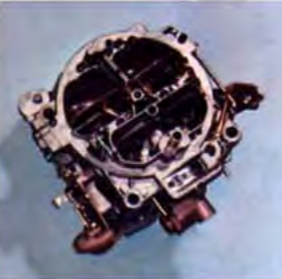
New Quadrajt Carb. 40% increase in capacity through air-metered secondary throttle bores. Primaries with smaller venturis for added economy.
