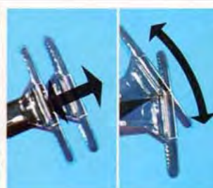
Tilt-and-Telescope Steering Wheel —Adjusts up-and-down to seven positions, in-and-out up to 3 inches. Available on all models except F-85. Tilt-Away Steering Wheel moves up and down, is optional on F-85 only.
