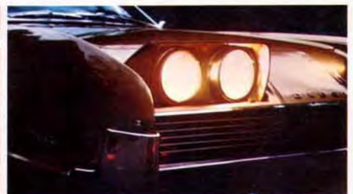
Smart, concealed headlamps open up in seconds when lights are turned on . . . retract automatically into low-slung Toronado hood when lights are turned off.
