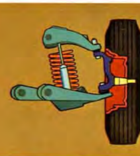
Pivot-Poise Front Suspension keeps Olds "steady as she goes!" "A" frame upper and lower control arms with wide pivot points combine with extra-wide wheel tread to improve stability regardless of road conditions.
