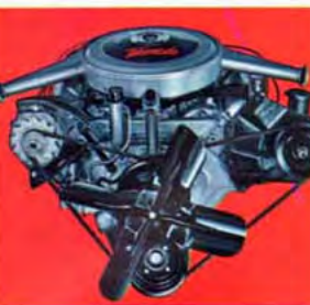
Oldsmobile's most powerful V-8! 425-cu.-in. Toronado Rocket Engine delivers 385 horsepower.
