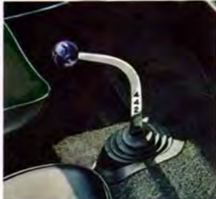
Four-on-the-floor. Stick shift, fully synchronized, extra cost. Fully synch 3-speed with column shift, standard. (Floor-mounted, extra cost.)
