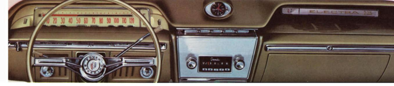
Instant instrument viewing. With Buick's Mirromagic instrument panel you see all instruments in a tilted mirror without glare or reflection.
