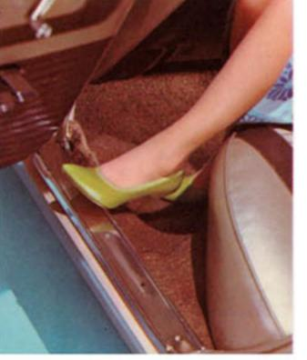
The dogleg is gone from the front door entrance to provide nearly five inches more of diagonal entry room. Door sills are narrower, too, for easier getting in and getting out. And Buick's new Hide-Away Drive Shaft reduces the tunnel height to give the middle passenger more leg room to stretch out and relax.
